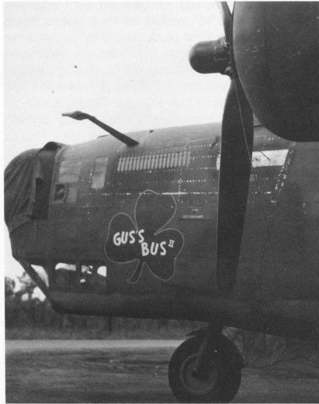
#125 Gus's Bus II nicely illustrating the Oklahoma City modification Ed Loy Collection
