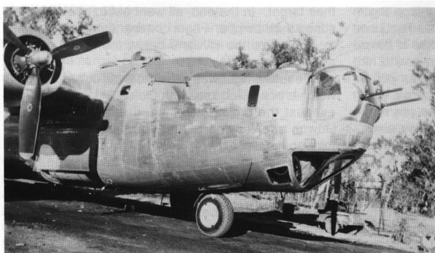
Between missions at Darwin. Note the variations in this "J" model B-24: A6B hydraulic nose turret, the lack of a pitot tube on the right side and the bombardier side windows.
