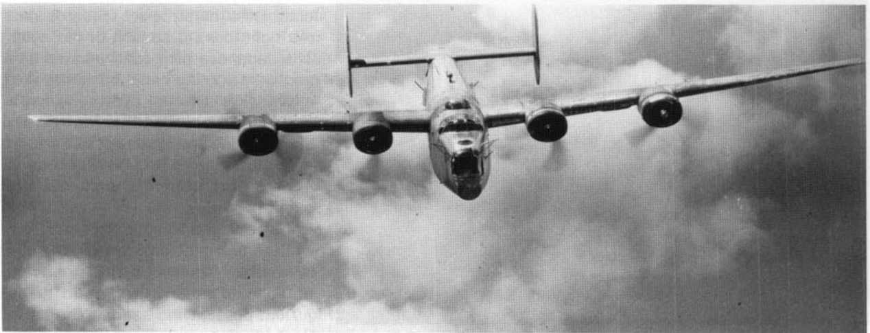
A "J" model B-24 with braced pitot tubes and hydraulic nose turret. Dexter Baker Collection
