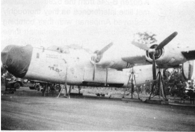
#134 Milady up on jacks for some landing gear work. William Camp Collection
