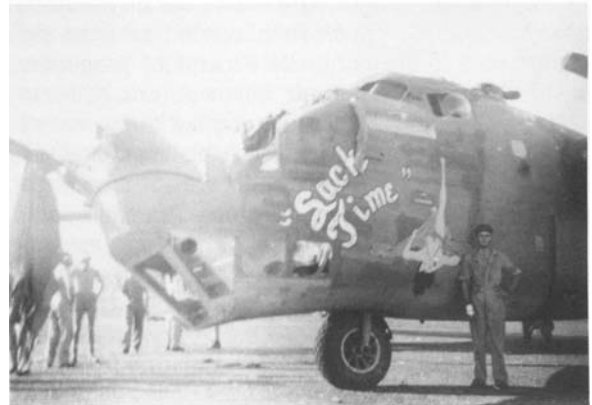
Although obviously askew, this photo gives the reader a good idea of what the Oklahoma City turret modification looked like installed on "D" model B-24s.
