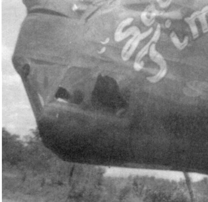
View of Nose Window Damage
