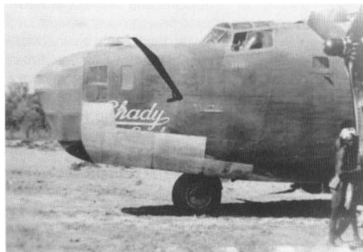
Damaged nose turret modification removed and old "greenhouse" put in place; she was on her 5 th mission when this damage occurred.
