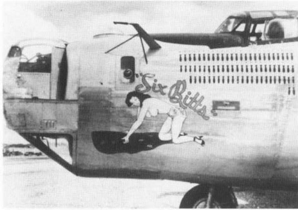
#214 with its A6B turret, braced pitots and no bombardier side windows. Don Sheets Collection
