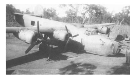
JEZEBELLE, B-24D-170-CO, 42-72953 of the 529<sup>th</sup> Squadron. This ship was damaged at Long Strip when someone turned too tightly trying to taxi out of the revetment.
