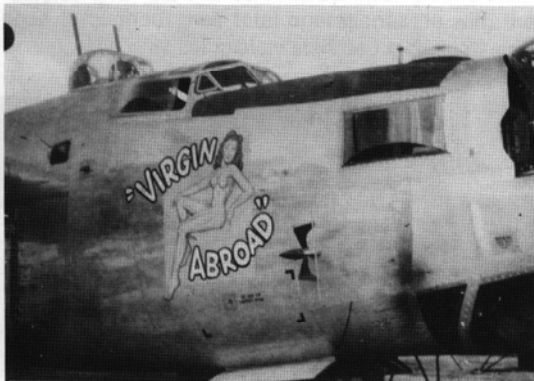
The 529th's #792 Virgin Abroad , a B-24M-10-FO from Willow Run showing the "high hat" top turret, elongated navigator side windows, triangular ones in the bombardier's compartment, Emerson nose turret plus a radar jamming antenna. Robert Withom Collection
