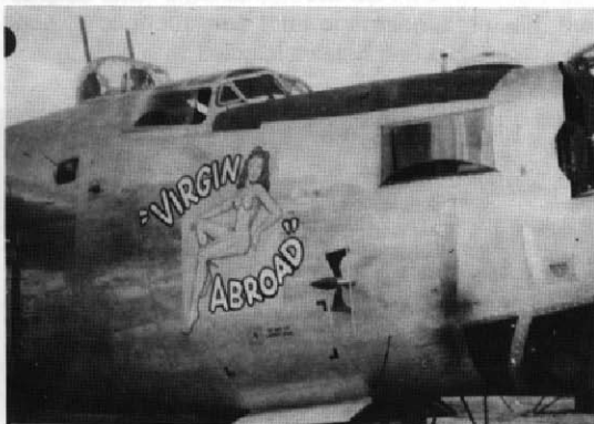
The 529th's #792 Virgin Abroad , a B-24M-10-FO from Willow Run showing the "high hat" top turret, elongated navigator side windows, triangular ones in the bombardier's compartment, Emerson nose turret plus a radar jamming antenna. Robert Withorn Collection
