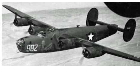
TEMPERAMENTAL DUCHESS (42-6982): Example of a Ford B-24E; this one was used as a trainer. The three last digits of the serial number on the nose invariably identify a plane as a training aircraft in the U.S.
